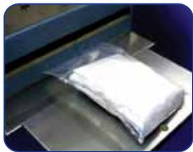
Product ready to be sterilised, is packed in a polyethylene bag.
