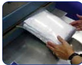
EtO is injected into the bag that is then automatically heat sealed.
